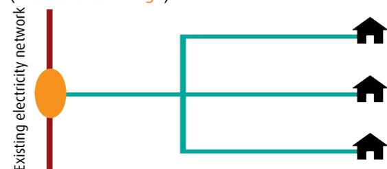
If **Option C** is accepted, your appointed ICP will be responsible for the installation of the new network, including final connection, at either LV or HV (indicated in green).
